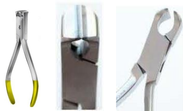
End Cutter For Hard Wire 145mm Tungsten- Carbide Insert MAX 1.0mm (.040")
